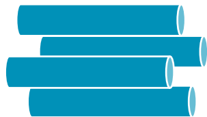
Quadrupole Mass Filter (Q1) Selection of Parent Compound
